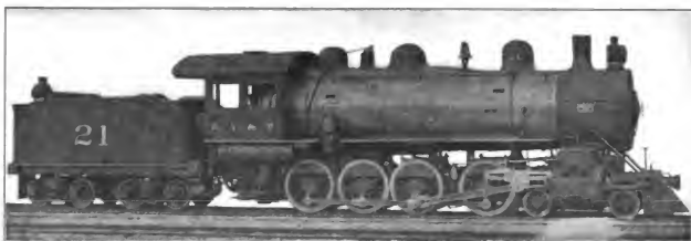
Fig. 72. Twelve-Wheel (4-8-0) Cross-Compound Locomotive. Built by the American Locomotive Co. for the Butte, Anaconda & Pacific. Cylinders 23 in. and 34 in. x 32 in., Working Steam Pressure 210 lbs. per sq. in., Total Heating Surface 3,806 sq. ft., Diameter of Drivers 56 in. Weight on Drivers 166,900 lbs., Total Weight 216,500 lbs.
